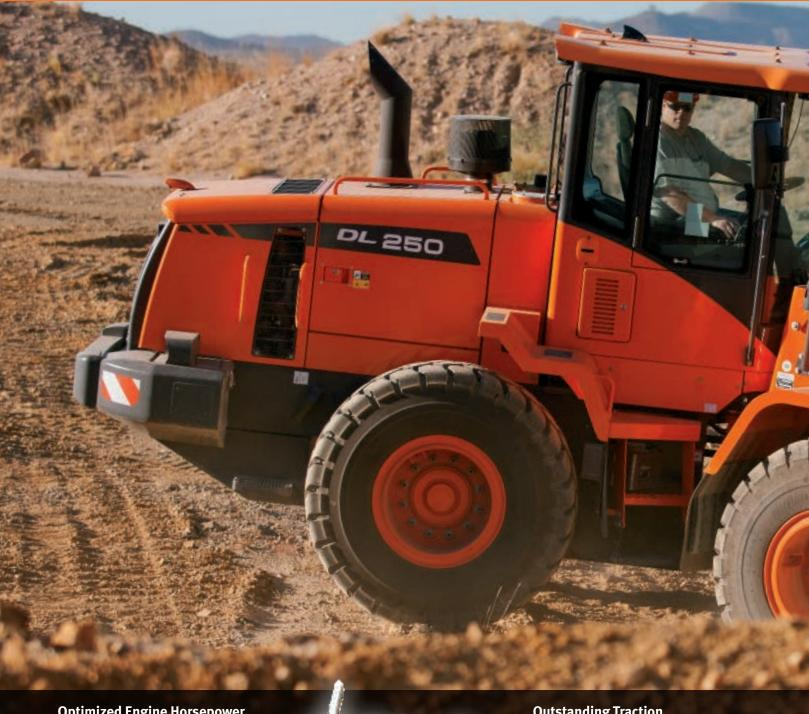
Optimized Engine Horsepower A finely tuned horsepower curve and increased torque ensure you can move mountains of material fast. A high pressure common rail fuel injection system and Cooled Exhaust Gas Recirculation (CEGR) valve reduce emissions.
