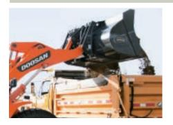
With a sloped bottom for maximum filling and material retention, this is the perfect bucket for day-to-day material handling. Capacities range from 4 to 6.5 yd<sup>3</sup>.
