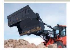
Leveling, dozing, digging, grappling, loading and dumping—this multi-purpose bucket is ready for whatever you've got. Capacities from 3.5 to 4 yd<sup>3</sup>.
