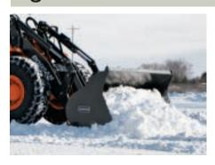
When you need to move snow, mulch or other light material in a hurry, the light material bucket is the economical choice. Comes standard with bolt-on cutting edge.
