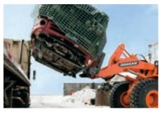
Easily lift, carry and place materials. Pallet forks with 48" or 60" forks available for DL200-3, DL200TC-3, DL220-3, DL250-3 and DL250TC-3 wheel loaders.
